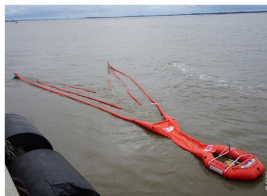
Photo 29 Trial in Loire estuary of a floating hydrocarbon containment and collection system for fast current-LMOS Sweeper system- (source Cedre)
