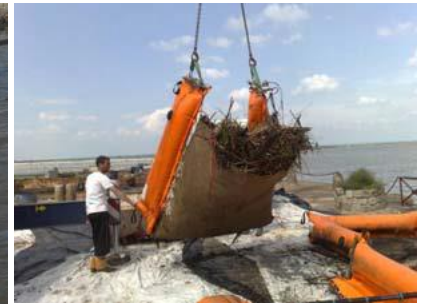
Photo 21 Craning a Thomsea trawl full of polluted floating reeds (source Thomsea)
